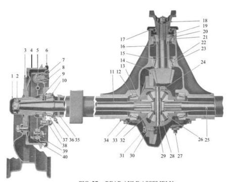
FIG. 27 -- REAR AXLE ASSEMBLY (Semi-Floating Type)
